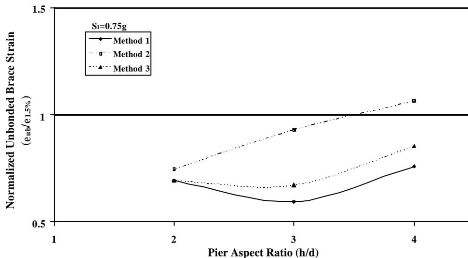
Figure 9. Observed strain demands normalized by target strain of 1.5%.
