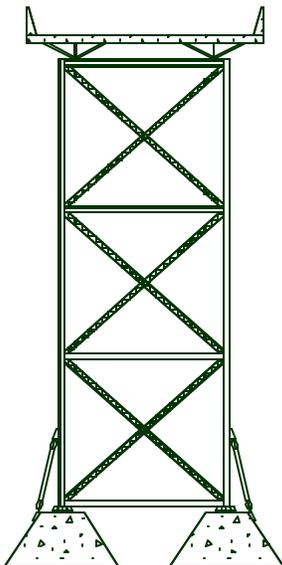
Figure 2. Sketch of retrofitted pier.
