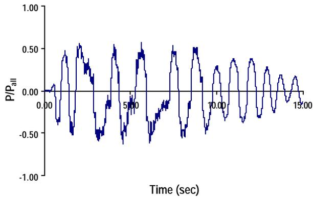
Figure 13. Horizontal base shear.
