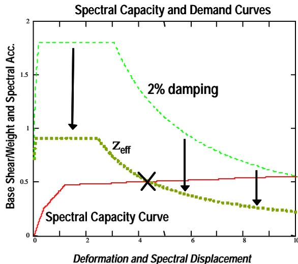
Figure 8. Capacity spectrum plot.
