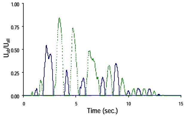
Figure 12. Uplift at foundation.
