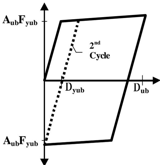
Figure 6. Unbonded brace response.
